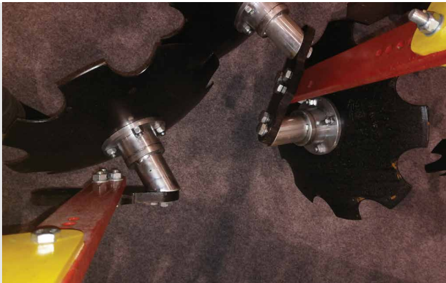
Sheet metal shield + RS seal/Dirtblock seal + Forged cover plate
